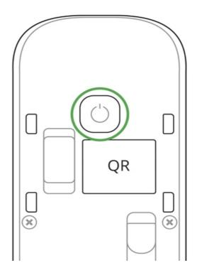
For the detection and interfacing to occur, the detector should be located within the coverage area of the wireless network of the hub (at a single protected object). Request for connection to the hub is transmitted for a short time at the time of switching on the device.
