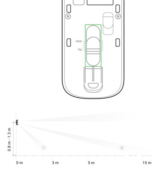
The lower PIR sensor beam direction with the specified minimum (1) and maximum (2) detection range
